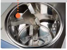
Provided with eccentric blades, the only one without central shaft to mix homogeneously and continuously any ingredient without stressing product texture, especially pastry cream during its cooling and storage.
