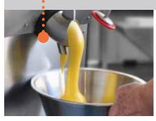
Single-block steel body, seamless for a perfect product output. Double safety device and variable diameter for a quick and easy outgoing of both liquid products such as mixes and very dense products such as cream at + 4°C. After each dispense the exceeding product goes back into the tank for correct storage and highest hygiene standards.
